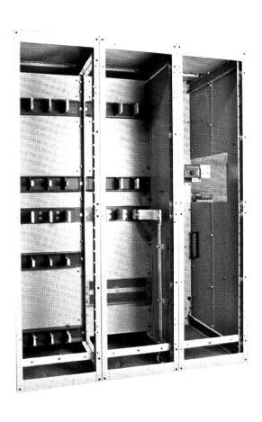
A combination of steel and glass polyester insulation isolates the incoming line from the main bus. This same combination of barriers can be specified to isolate the main bus from the cable connection area. This minimizes fault communication in these areas and affords safety to plant facilities and operating personnel.
