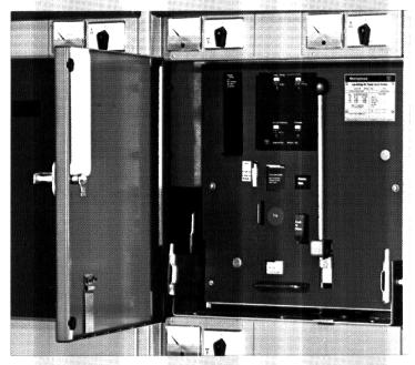
A rugged steel outer door with quick opening latches closes the compartment with the breaker in any position and provides a double steel barrier in front of the breaker. Even with the door open, a full sized metal shield on the breaker face assures that the breaker cannot be racked or operated without properly protecting the operator.
