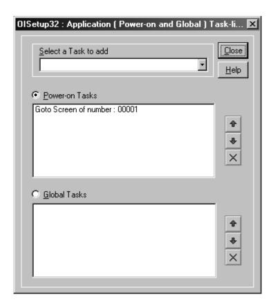
If user wants to control the screen display from the PLC, he must define a task 'Copy tag to STR' in Global task list. Now screens will be displayed depending on the value in the defined tag. Screens can also be changed from the touch key or conditional tasks in screen task list. Global task list need not include any 'Goto..' or 'Copy tag to STR..' task.
