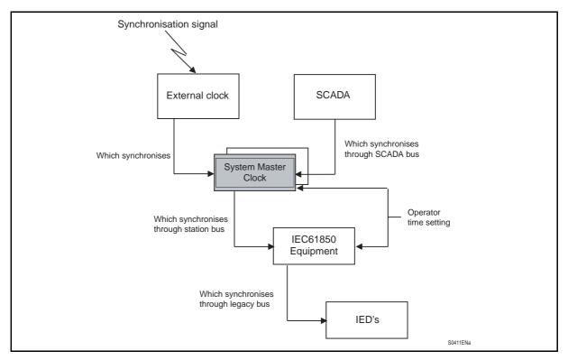
In case that external clock does not exist or is lost, the master clock equipment can be synchronised by a SCADA (only if the Master Clock computer manages a SCADA protocol) or by an operator. Synchronisation priority of the System Master Clock is in the following order:
