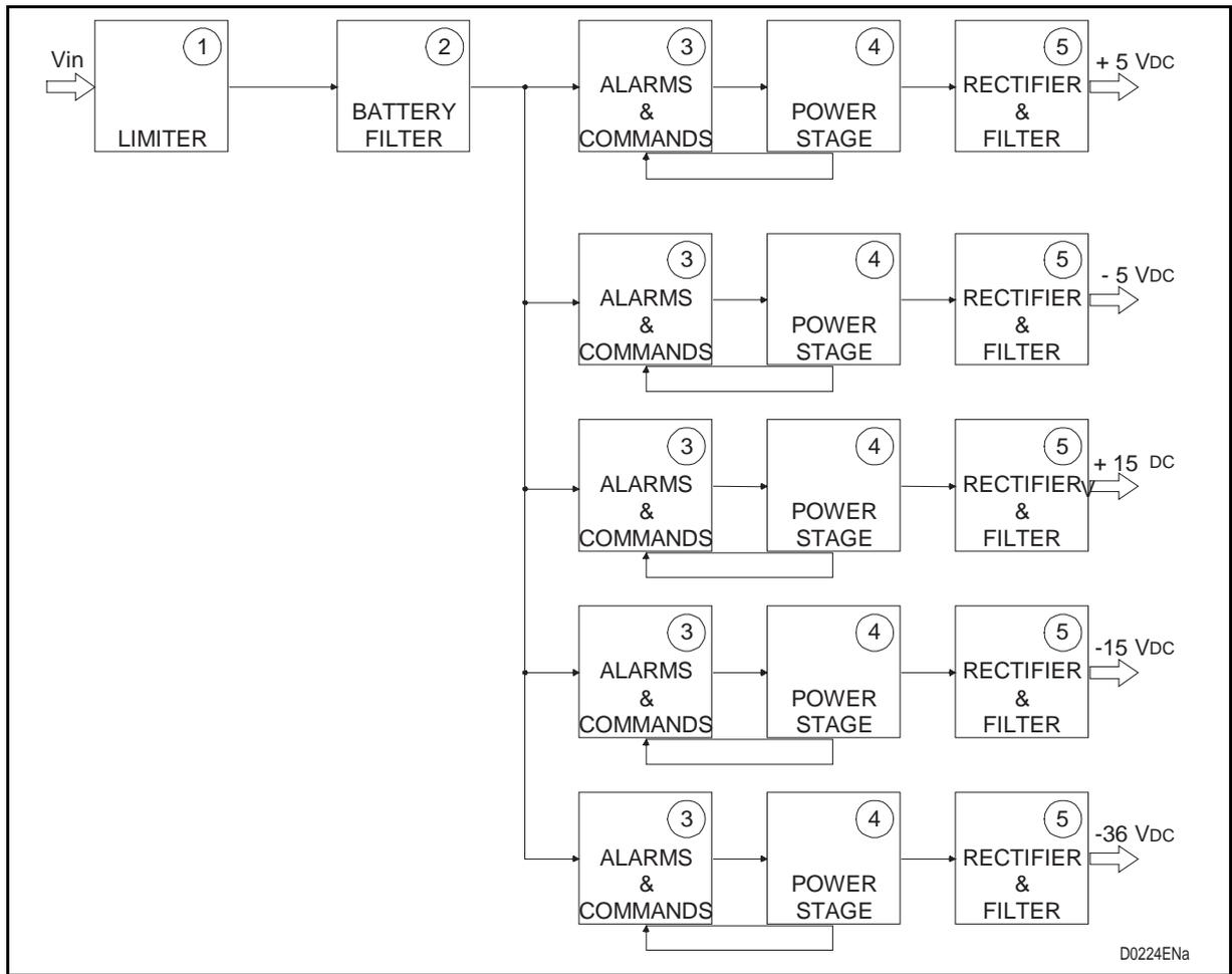
FIGURE 4 – POWER SUPPLY UNIT BLOCK DIAGRAM
