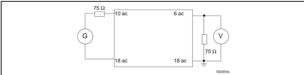
FIGURE 16 – TX FILTER TUNING TEST RIG
