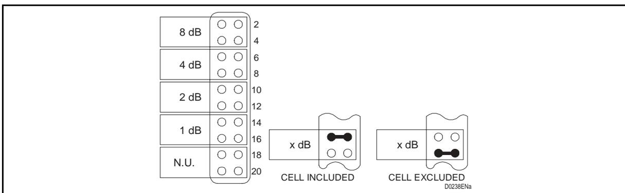
FIGURE 11 – INPUT / OUTPUT ATTENUATION CELL
