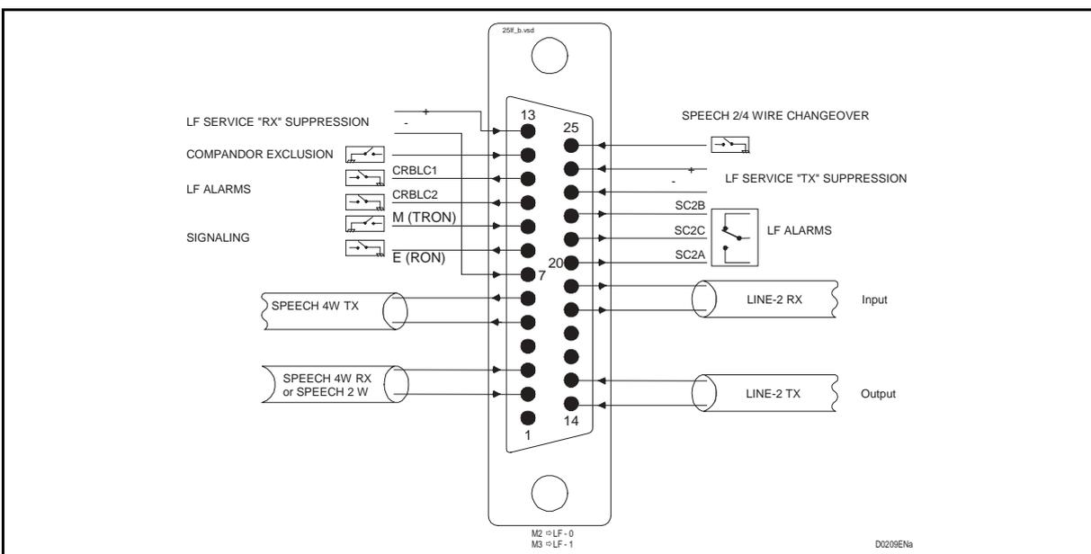
FIGURE 35 – LFS FIELD CONNECTOR M2 - LF0 OR M1 - LF1
