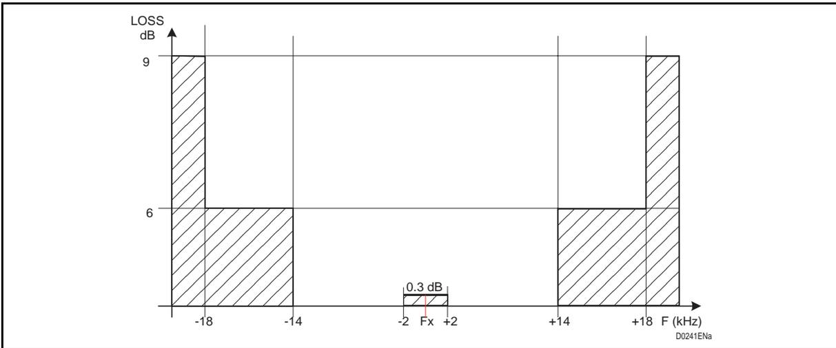
FIGURE 18 – FREQUENCY LOSS MASK FOR FC ≥ 396 KHZ-
