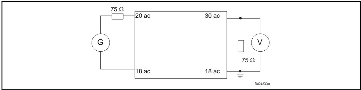
FIGURE 23 – RX FILTER TUNING TEST RIG
