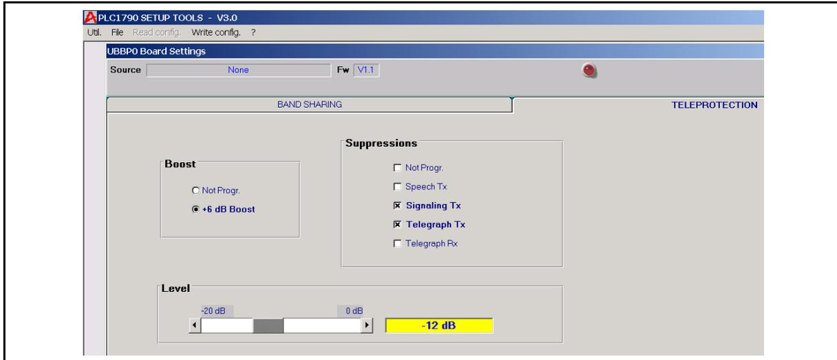
FIGURE 24 – UBBP TELEPROTECTION SETUP FUNCTIONS
