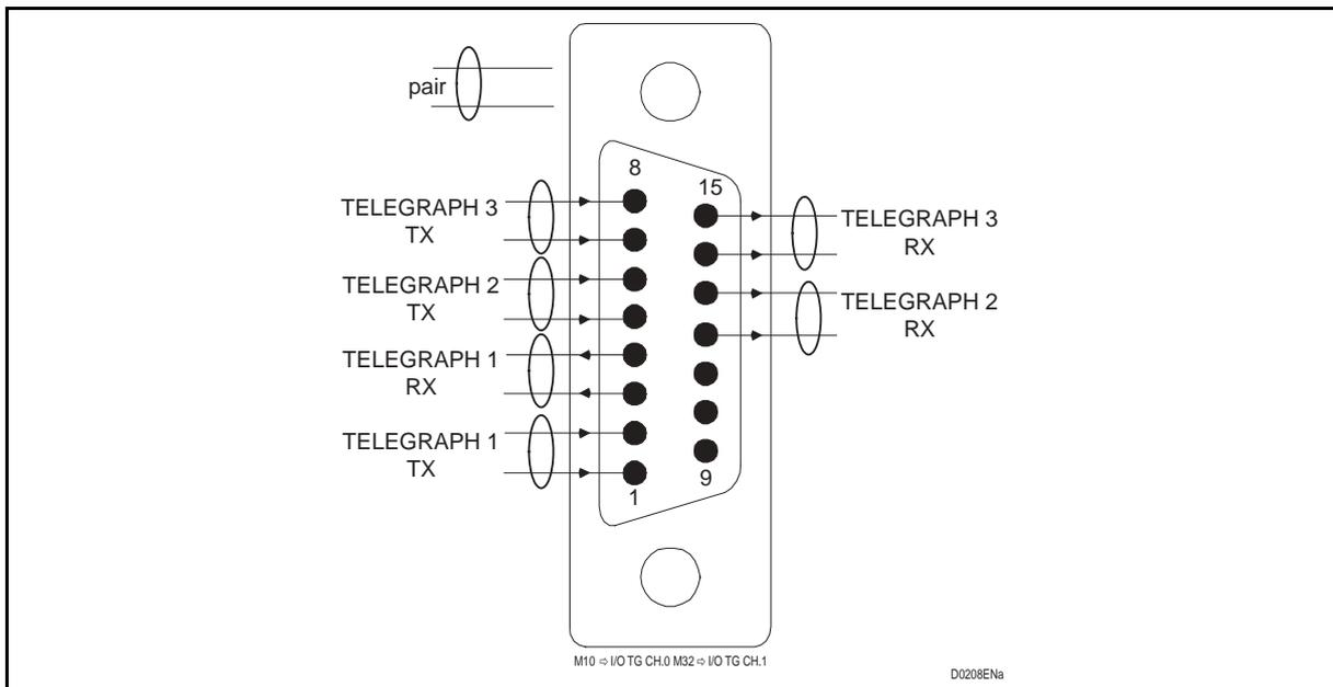
FIGURE 8 – INPUT / OUTPUT TELEGRAPH CHANNELS
