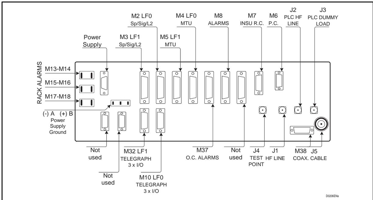
FIGURE 6 – FIELD INTERCONNECTION PANEL
