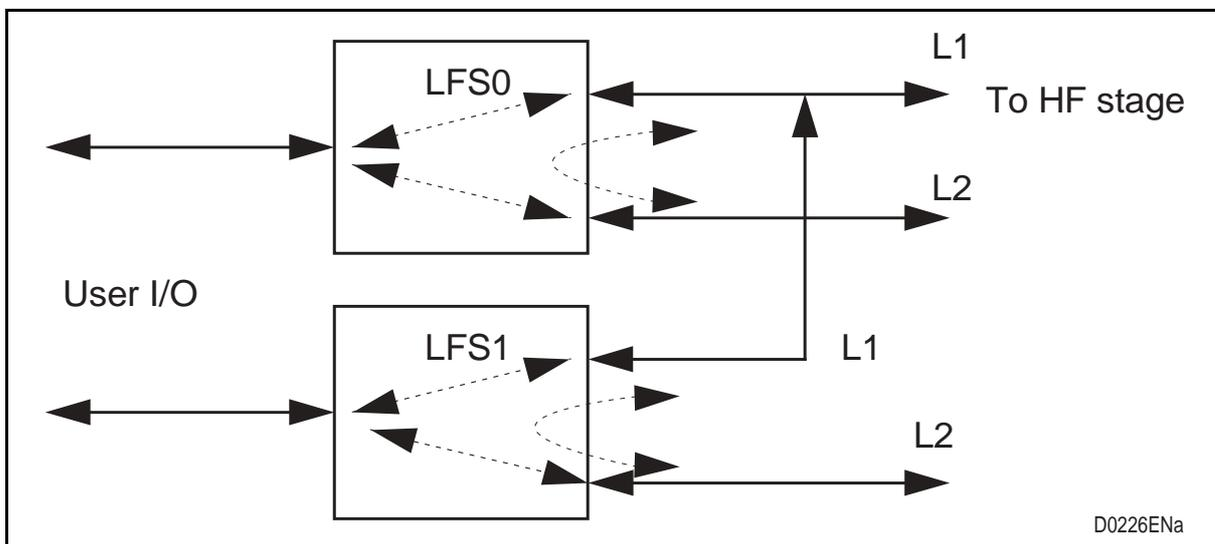
FIGURE 6 – COMMUNICATION CHANNEL WITH TWO LFS CARD
