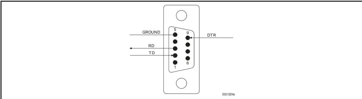
FIGURE 12 – M6 COMPUTER INTERFACE ( PROGRAMMING / MAINTENANCE )
