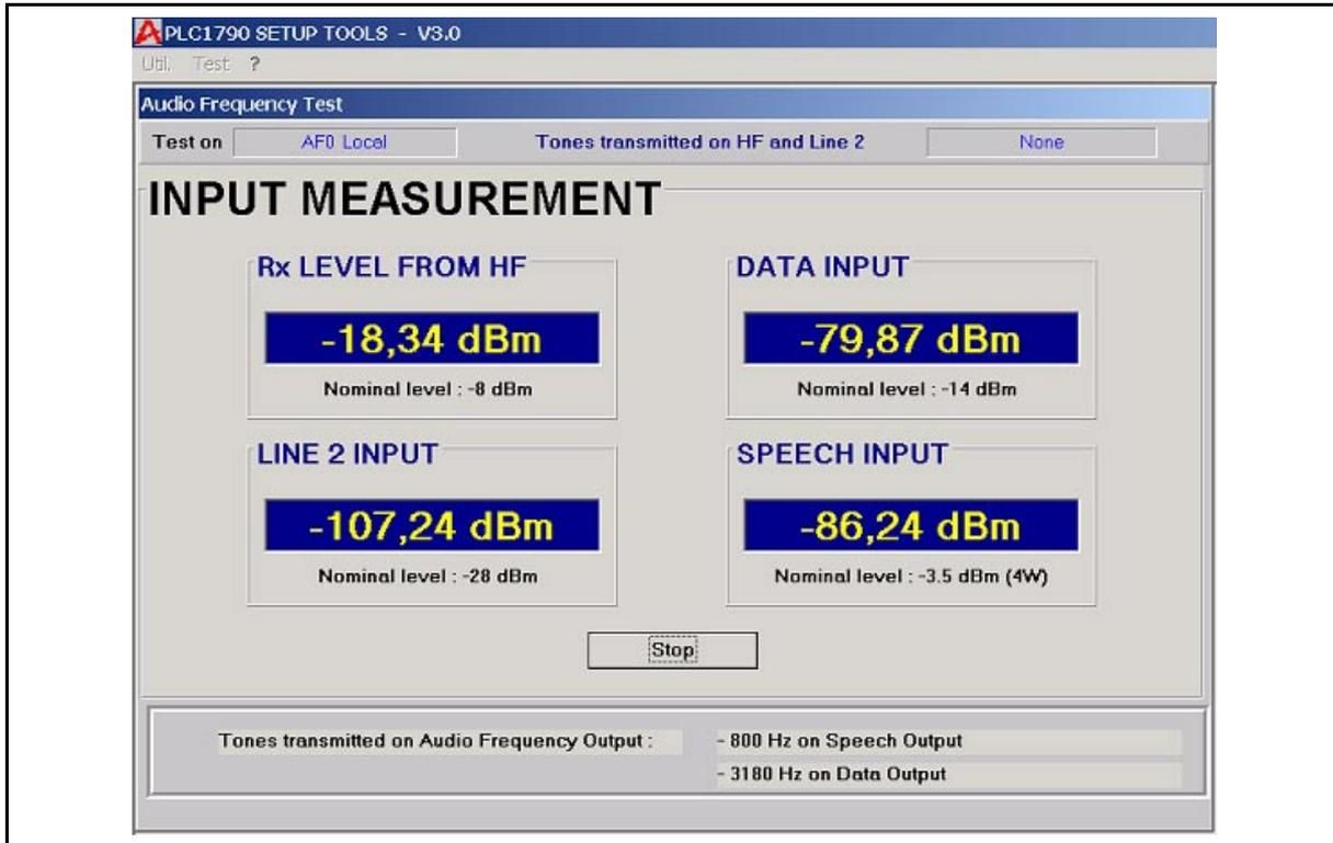
FIGURE 53 – LF INPUT SIGNAL MEASUREMENT WINDOW
