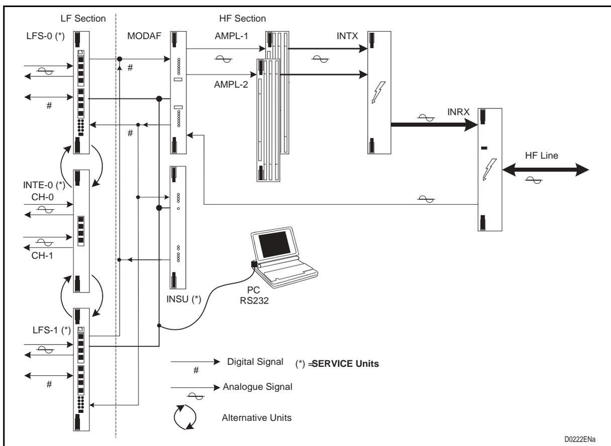
FIGURE 1 – PLC 1790/B REVISION2 FUNCTIONAL DIAGRAM
