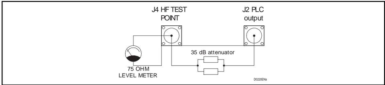
FIGURE 20 – HF TEST MEASUREMENT CONNECTORS
