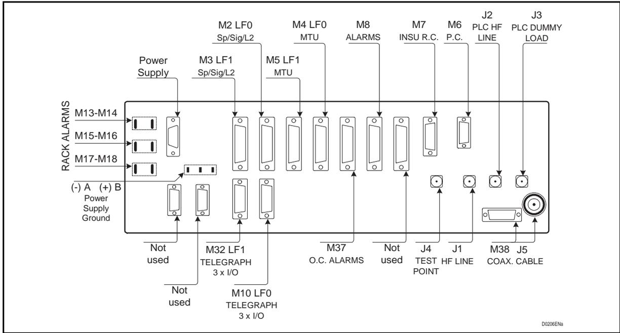
FIGURE 3 – FIELD INTERCONNECTION PANEL
