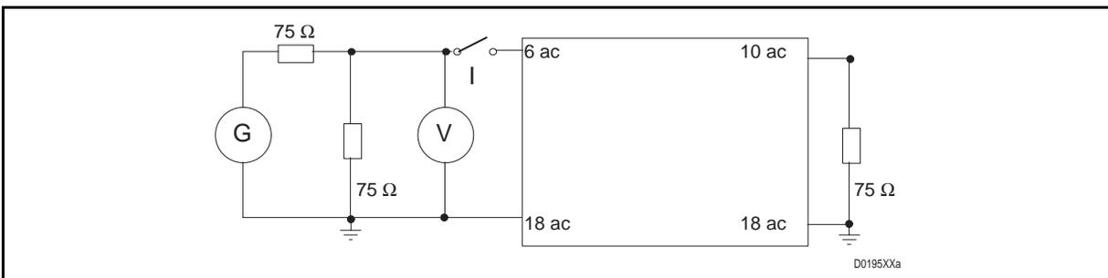
FIGURE 19 – TAPPING LOSS TEST RIG
