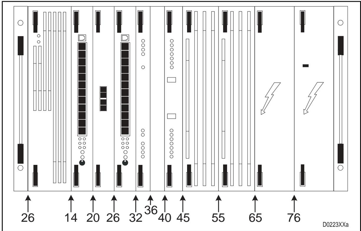
FIGURE 2 – PLC 1790/B REVISION2 SUBRACK - UNITS COMPOSITION
