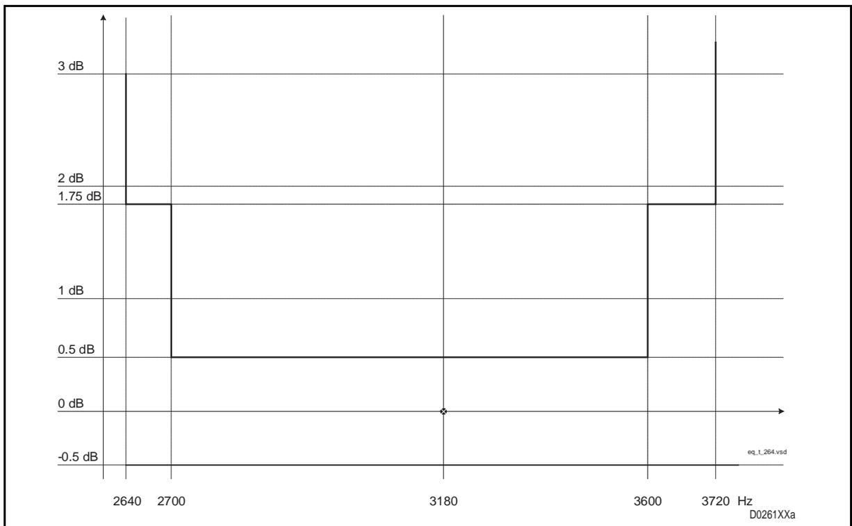
FIGURE 44 – TELEGRAPH CHANNEL 2640 ÷ 3720 HZ
