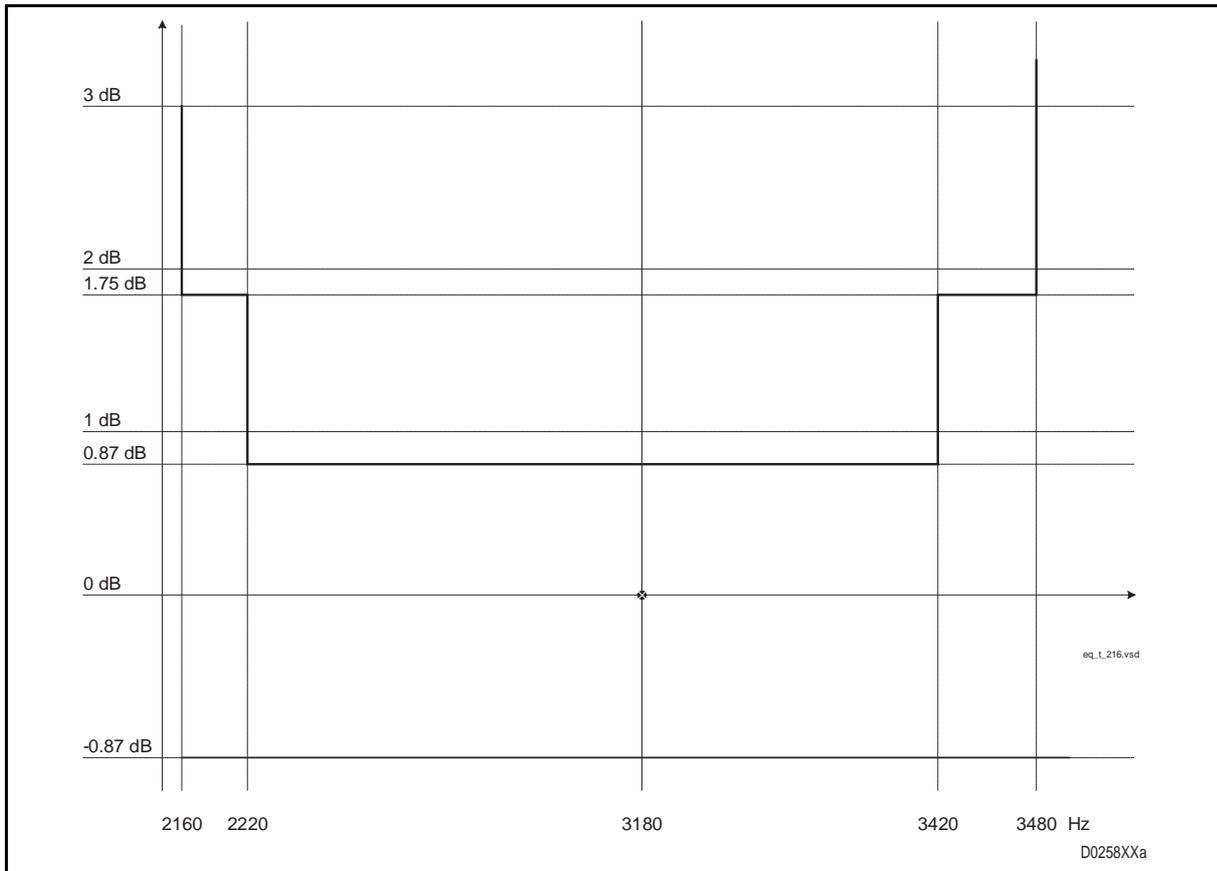
FIGURE 41 – TELEGRAPH CHANNEL 2160 ÷ 3480 HZ
