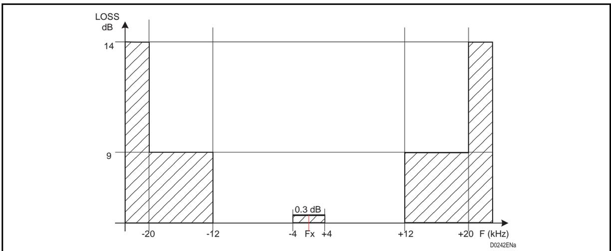
FIGURE 21 – FREQUENCY LOSS MASK FOR  $FC \geq 400$  KHZ
