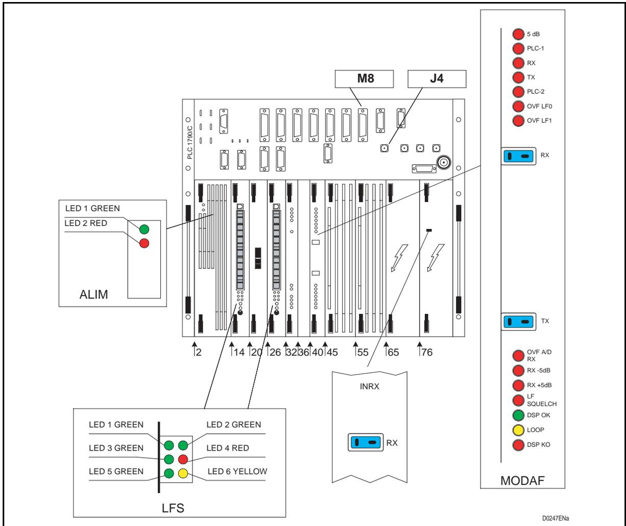
FIGURE 27 – PLC LED'S AND TEST POINT
