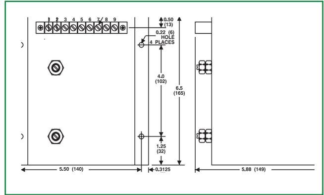
FIGURE 3. SENSING MODULE OUTLINE DRAWING
