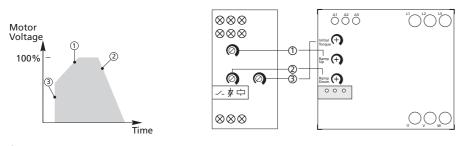
1 Ramp-up time. Time from zero load voltage to full load voltage.
