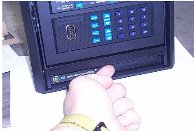
Figure 3-5: PRESS LATCH UP AND PULL HANDLE
