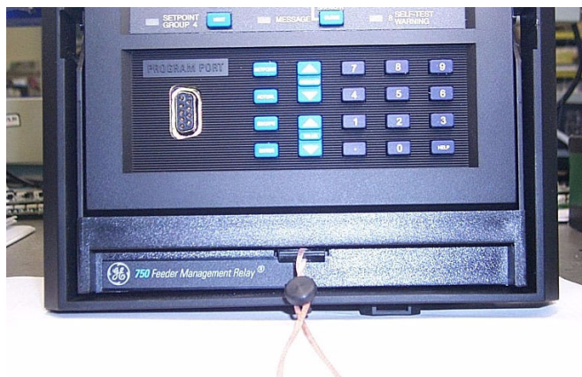
Figure 3-2: DRAWOUT CASE SEAL
