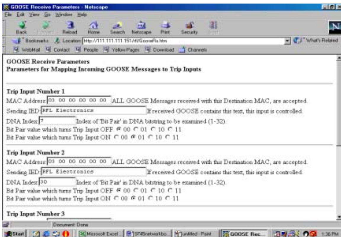
Figure 10-13. GOOSE Receive Parameters Setup
