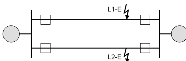
Figure 2-5 Multiple fault on a double-circuit line
