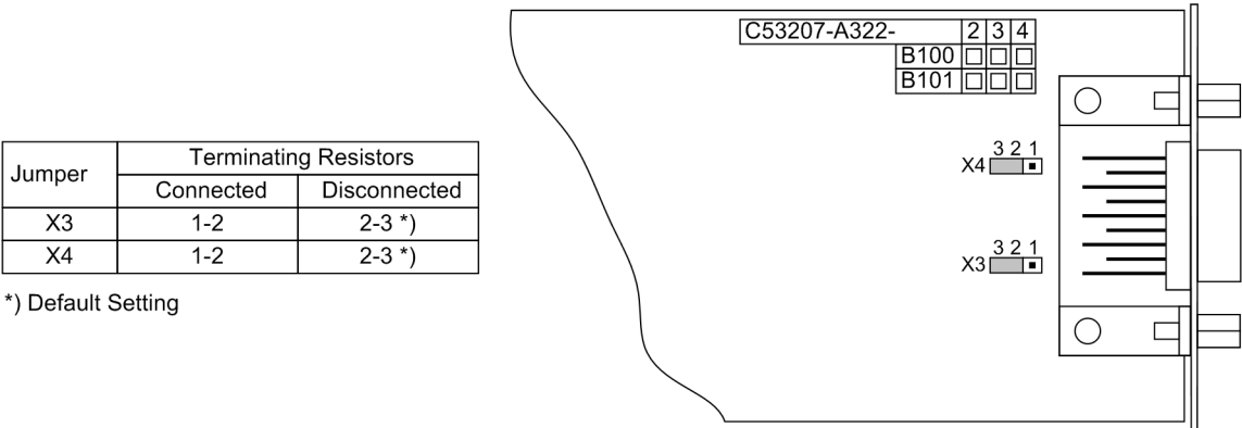
Figure 3-13 Location of the jumpers for configuring the terminating resistors of the active electrical module (PROFIBUS and DNP 3.0 interface)
