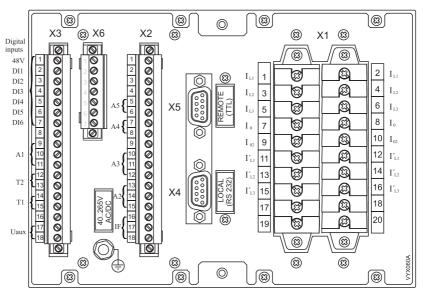
The generator, transformer and motor differential protection relay is connected to the protected object through the following measuring and control connections:
