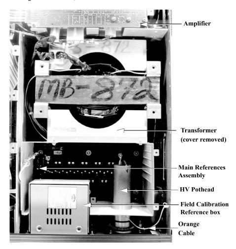
Figure 4.27 M4100 Chassis, Covers Removed
