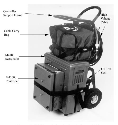
Figure 1.9 M4000 Insulation Analyzer in Storage Mode
