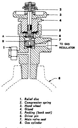
Fig. 3. Gas cylinder valve shown in closed position
