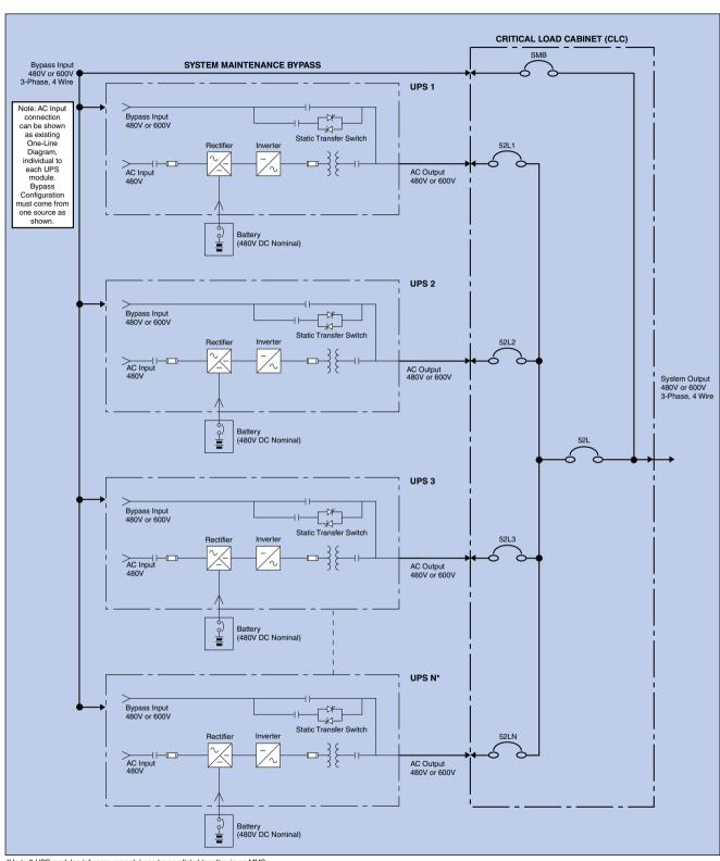
\*Up to 8 UPS modules (of same capacity) can be paralleled together in an MMS.
